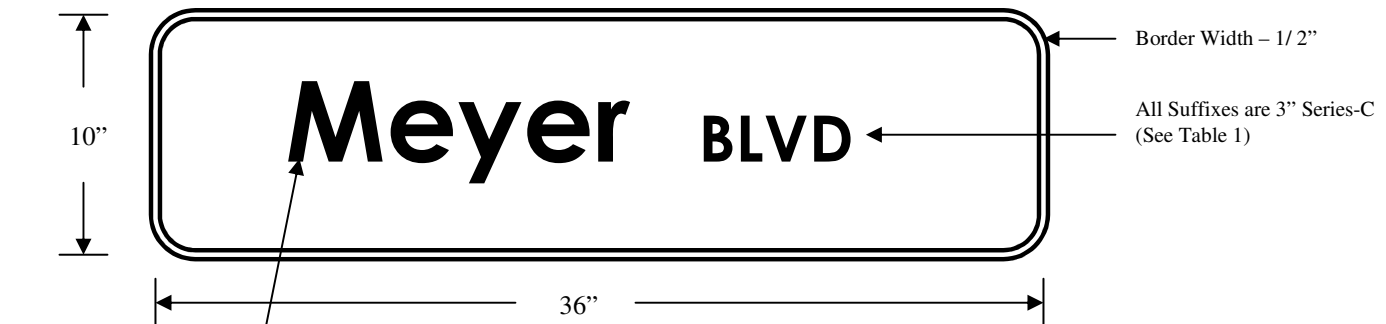
TYPICAL LAYOUT FOR NON-GRID STREET NAME SIGN
