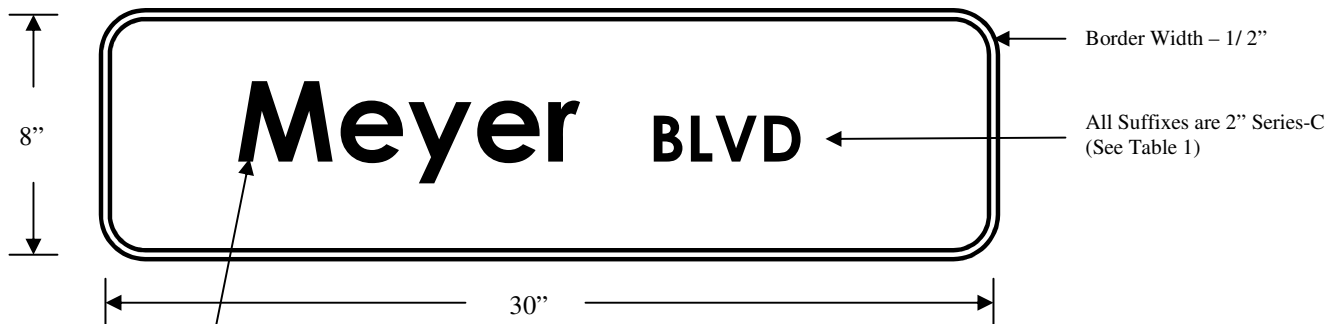
TYPICAL LAYOUT FOR NON-GRID STREET NAME SIGN
